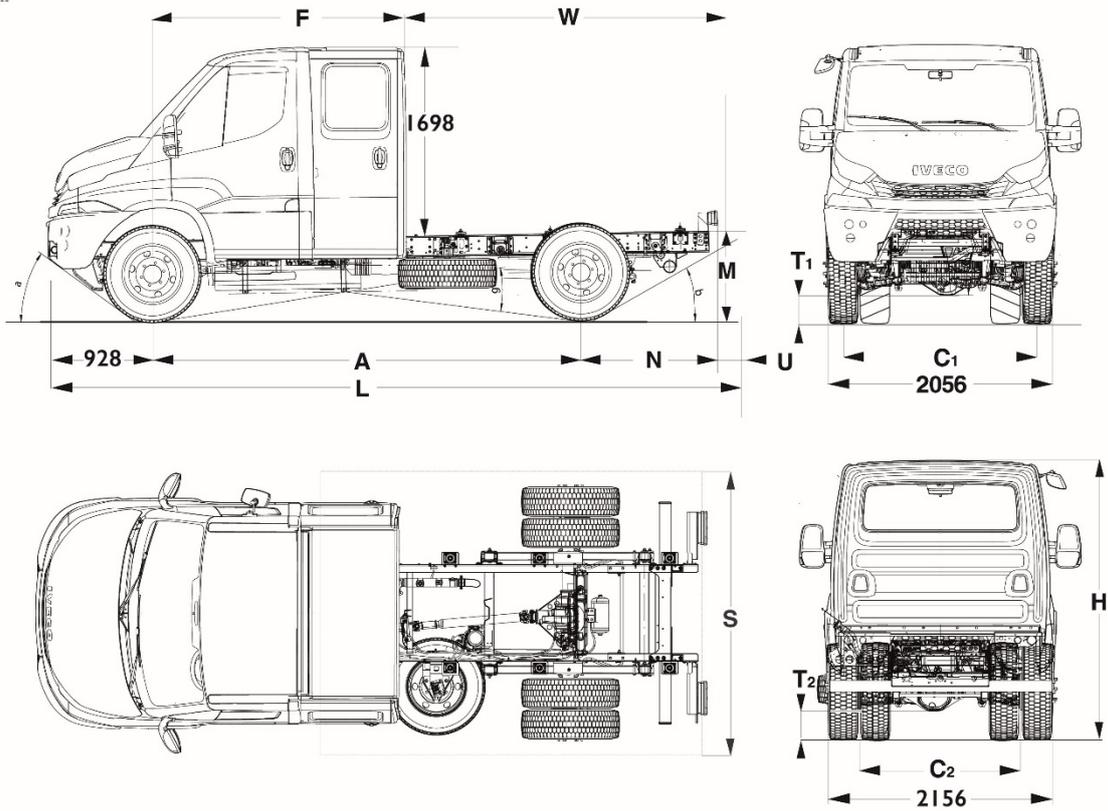
**ABMESSUNGEN (in mm)**
